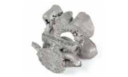
Rough casting due to overheating
