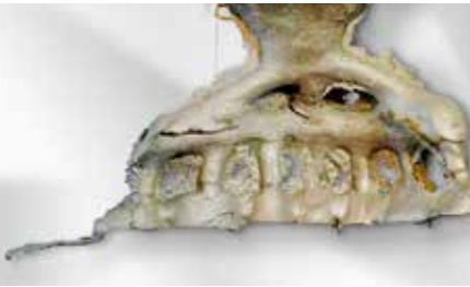
Casting flash on casting
