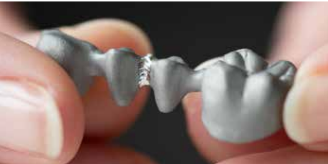
Laser weld seam
