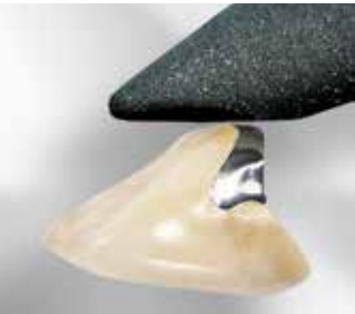
Fig. 4 · Rubbering as prepolishing
