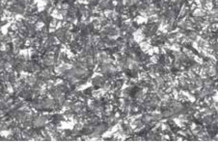
Wirobond® 280 blasted with Korox® 250 µm
